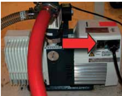
Figure 1. Vacuum pump power switch
